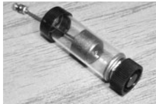
Figure 2: Close-up of Airpot without rubber casing
