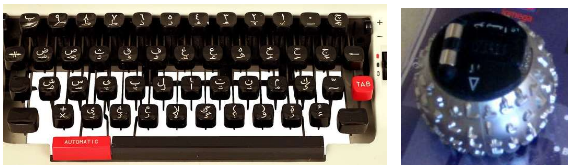
Fig. 11. An early Persian typewriter keyboard and IBM Selectric golf-ball print mechanism for Persian.
