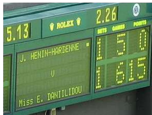
Fig. 18. Early dot-matrix displays were used at airports and on stadium scoreboards.
