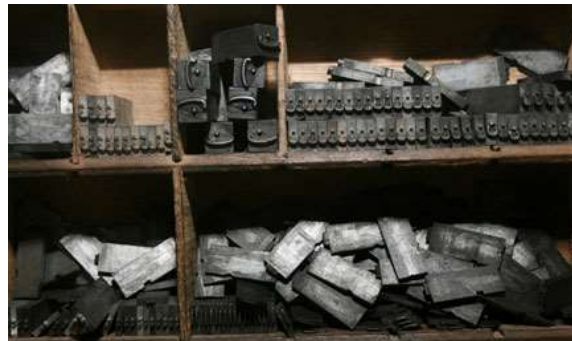
Fig. 6. Movable Persian type in the compartments of the typesetter's tray.
