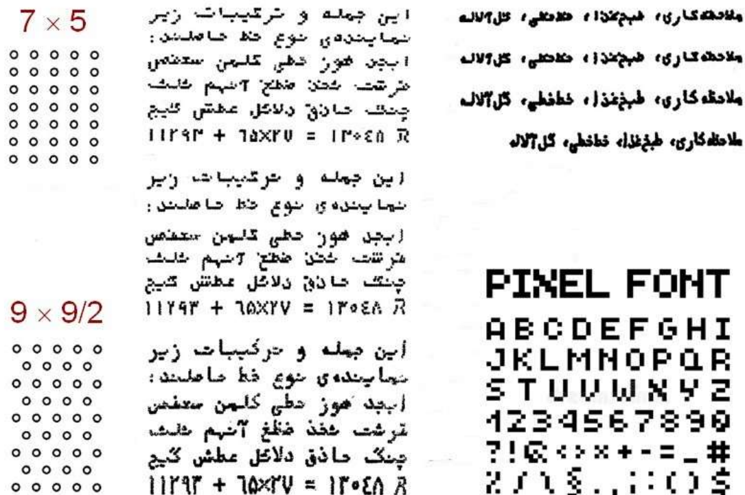
Fig. 28. Some results of a study to determine the minimum dot-matrix size for Persian script..
