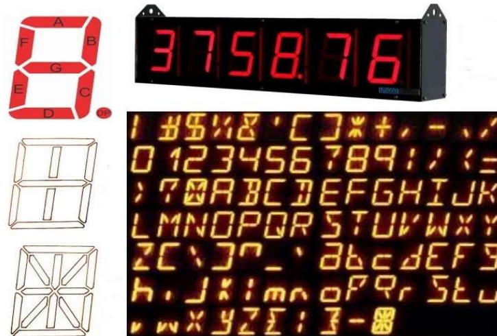
Fig. 16. Line-segment display devices for numerals, Latin alphabet, and special symbols.
