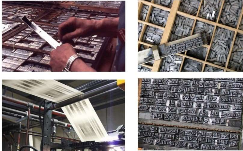
Fig. 4. Hand-typesetting with movable type, the tray holding the typeset text, and the printing process.
