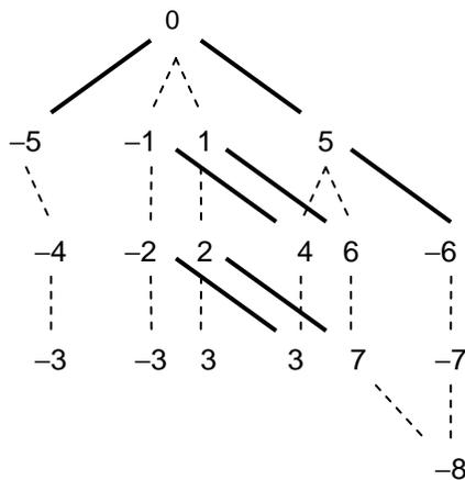
Fig. 3. A graphical depiction of some shortest paths from node 0 to other nodes in  $CR(16; 5)$ . Solid and dotted lines represent chords and ring links, respectively.
