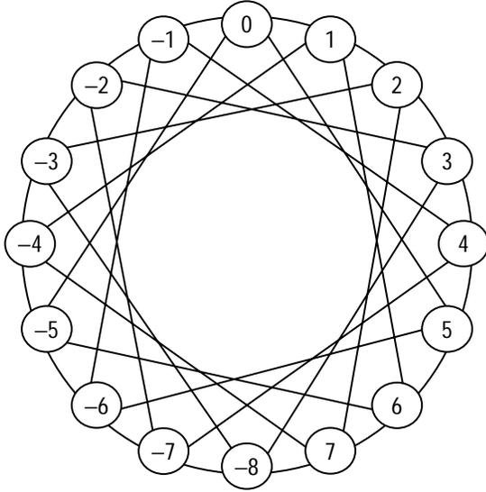
Fig. 1. The chordal ring network  $CR(16; 5)$  with 16 nodes and chord length 5.
