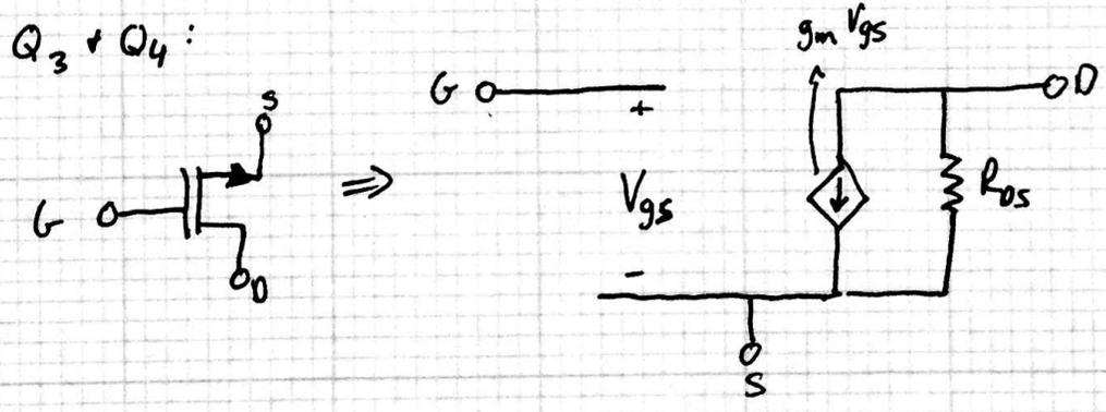
same as nmos b/c  $V_{gs} < 0$  changes direction of controlled current source ST  $I_0$  flows from Source  $\rightarrow$  drain
