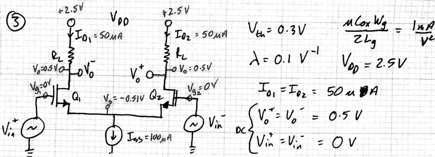
a)  $I_{SS} = I_{01} + I_{02} \Rightarrow I_{SS} = 100 \mu A$
