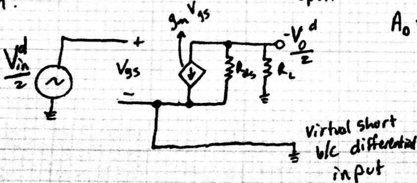
$$A_0 = \frac{V_{out}^d}{V_{in}^d} = g_m (R_L \parallel R_{ds})$$
