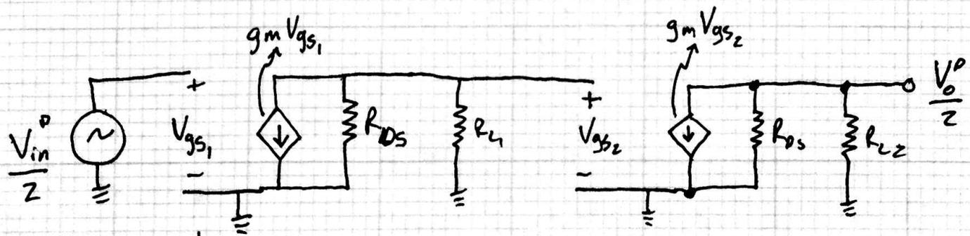
Stage 1:  $\frac{V_o^d}{V_{in}^d} = g_m(R_{ds} \parallel R_{L1}) = A_{V1} = 15.4$
