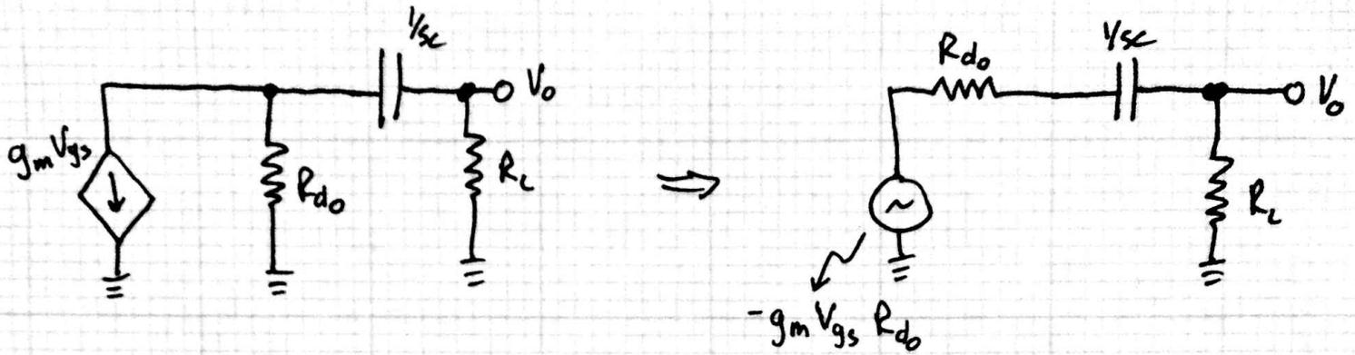
where  $R_{do} = R_{ds} \parallel R_d$
