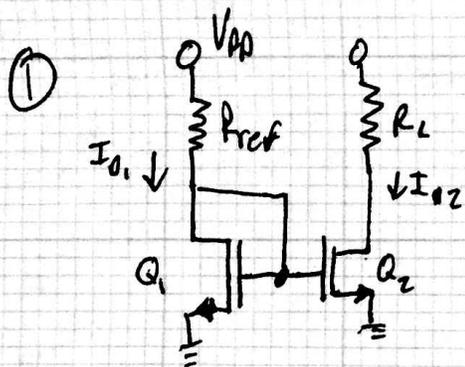
$$I_D = \frac{\mu C_{ox} W_{eff}}{2L_g} (V_{gs} - V_{th})^2 (1 + \lambda V_{ds}), \quad v_D > v_G - v_{th}$$
