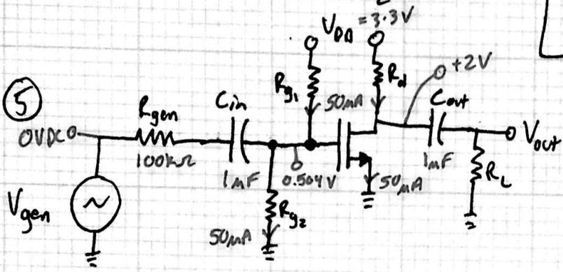
$$\frac{\mu C_{ox} W_g}{2L_g} = \frac{1\text{mA}}{V^2}, \quad \lambda = 0.1\text{V}^{-1}, \quad V_{th} = 0.3\text{V}$$
