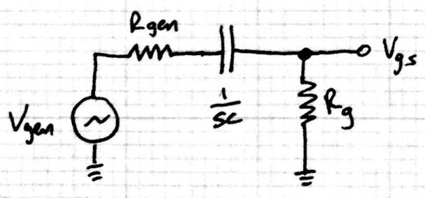
$$R_g = R_{g1} \parallel R_{g2}$$
