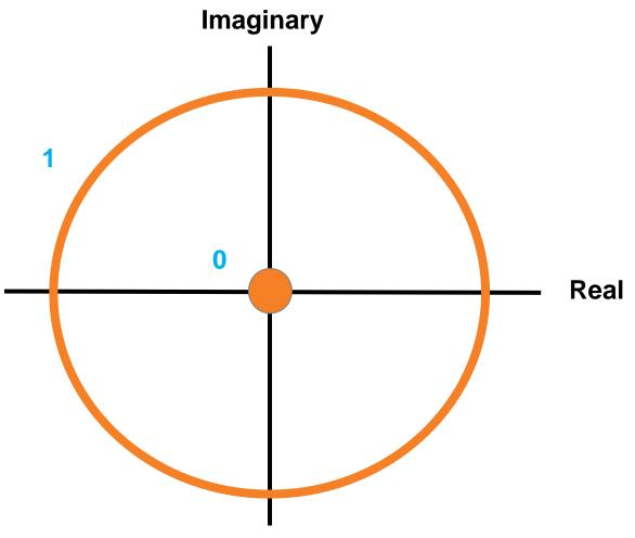
One bit encoded in the amplitude, per symbol 1 bit x 10 Gsymbols/second = 10 Gb/s
