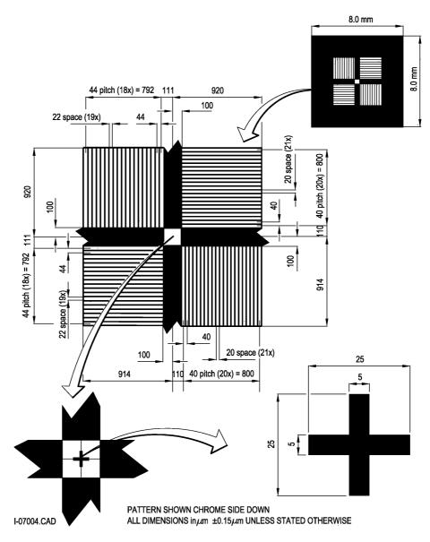
Figure 7.2 The reticle alignment mark
