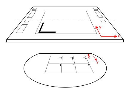
Figure 5.1 Relationship between reticle and wafer coordinate system
