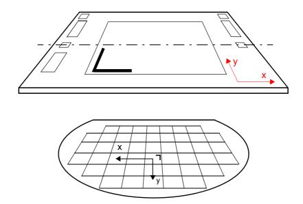
Figure 1.2 Relationship between reticle and wafer coordinate system
