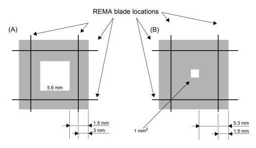
Figure 7.7 Examples of normal and extended image borders
