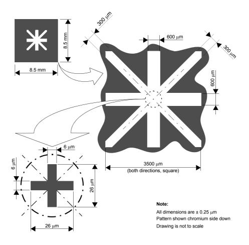
Figure 3.1 The reticle prealignment mark
