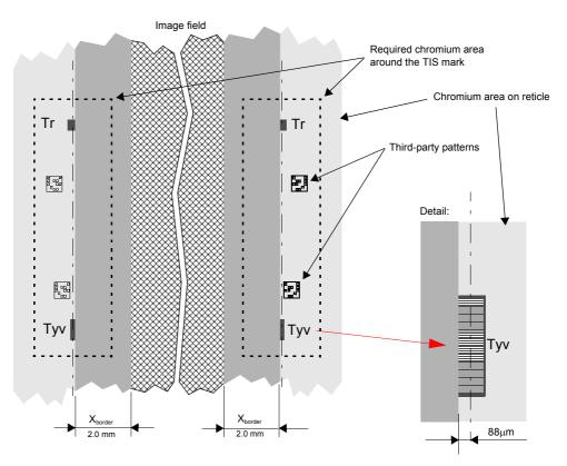
Figure 3.7 Example of various chromium borders (X direction) with TIS\_RSC-marks on the left and right side of the image field
