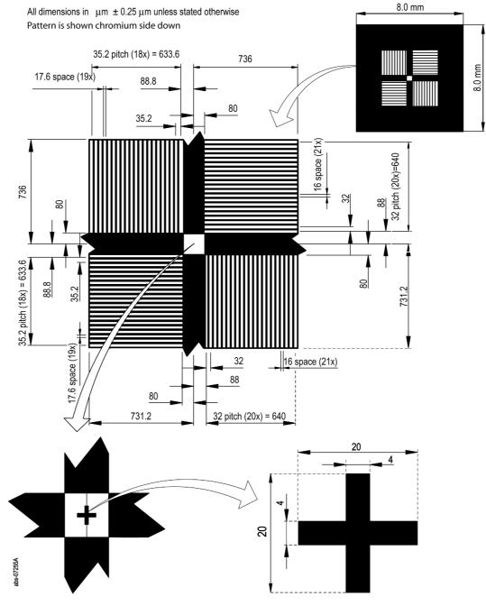
Figure 3.2 The reticle alignment mark
