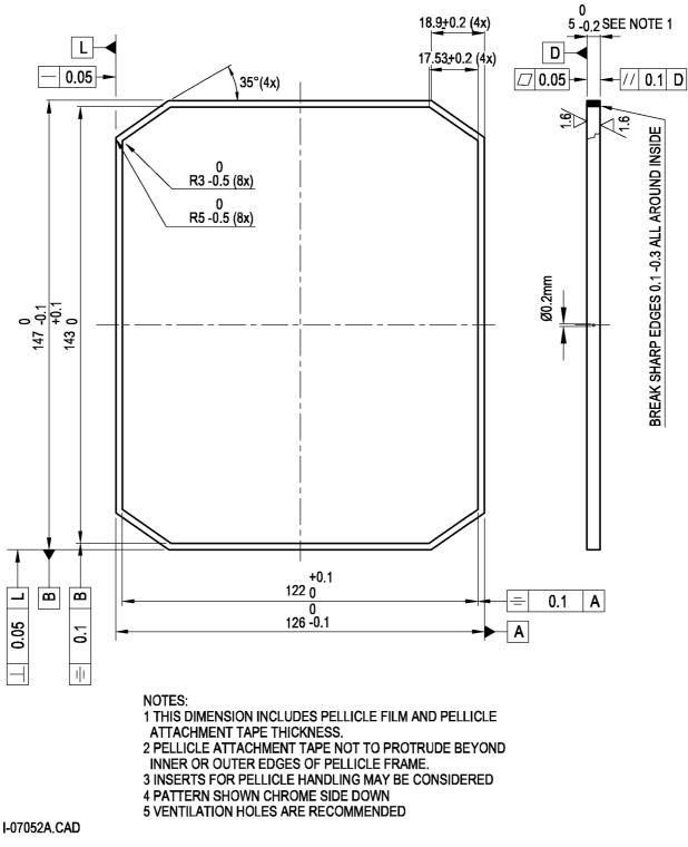
Figure 8.10 The recommended pellicle frame for PAS 5500/1xx series systems
