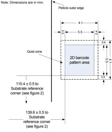
Figure 3.19 Details of location 'B' (right)
