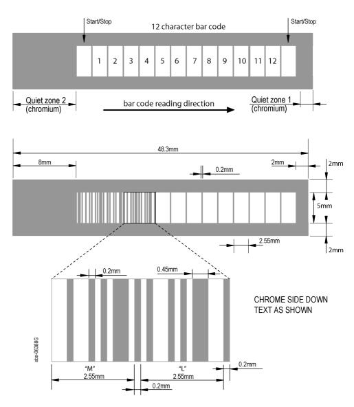
Figure 3.14 The bar code structure and dimensions
