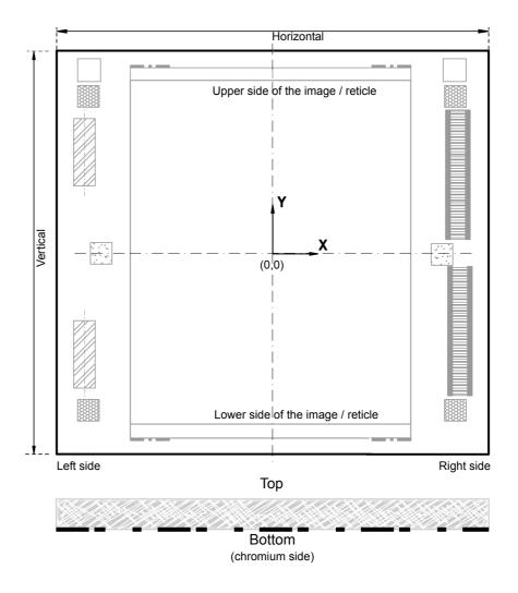
Figure 1.1 Definition of locations on a reticle
