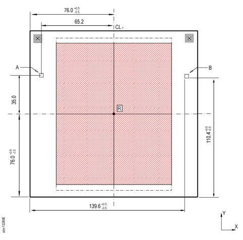
Figure 3.17 The two supported locations for a 2D bar code
