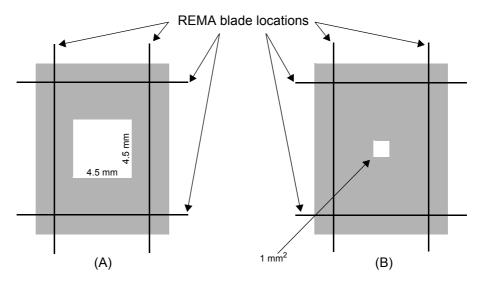
Figure 3.11 Example of a normal and extended image border (scanner situation)
