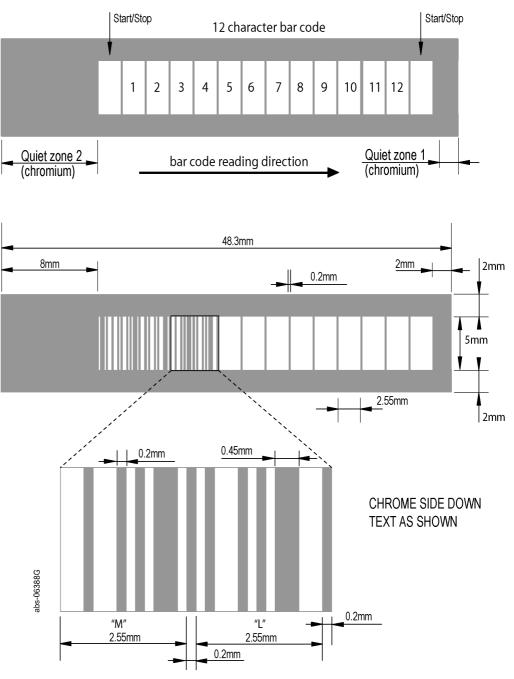
Figure 7.4 The bar code structure and dimensions
