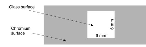
Figure 3.20 Release pin area
